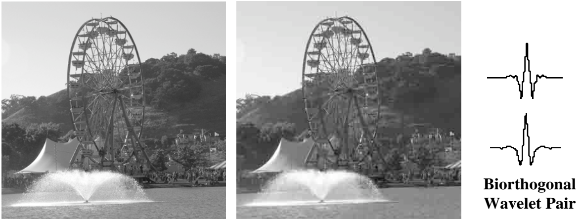
Figure 1.9-4 JPEG image compression of 91:1 achieved with a conventional DWT using a Biorthogonal 9/7 set of symmetrical wavelets.
